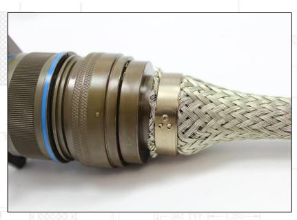
With the installation secured with the spring band and "Tri-Dent" protrusions located on the exterior of the spring band wrap, trim the excess braid.
