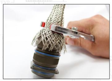
Using tooling pictured, compress the braid so that it conforms tightly to the profile of the banding platform. Moving radially, ensure that every portion of the banding surface has been formed uniformly.
