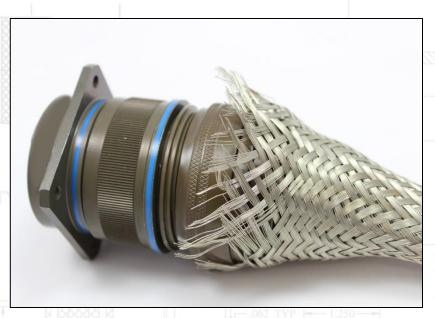
Pull braid over the banding surface of the connector accessory ensuring the braid overlaps the banding surface sufficiently and that there are no significant "windows" in the braid.
