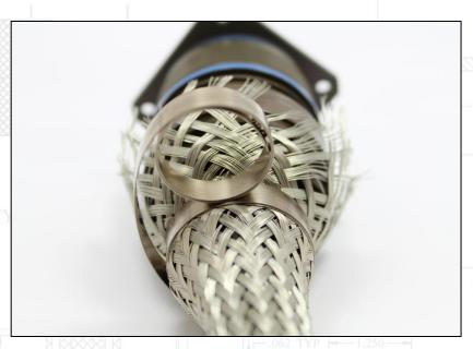
Begin to coil the spring band around the banding surface until the spring is completely coiled around the connector accessory and braid.
